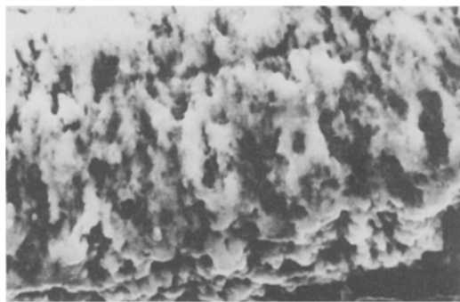
Fig. 2. SEM pattern of the cross-section of a stabilized platinum electrode (procedure II); f = 420 . \times 7000 .
